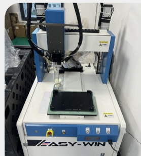
Automatic thermally conductive adhesive dispenser, to reduce the employees' health problems caused by the volatilization of chemical solvents.
