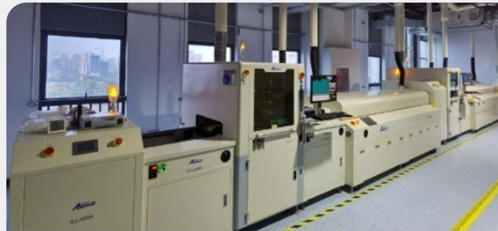
Fully automatic three-proofing coating line, to minimize employees' health problems resulting from chemical solvent volatilization
