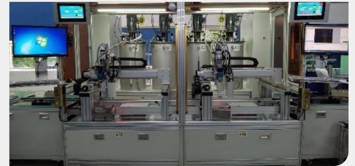
Fully automatic glue filling line, to improve glue filling stability and product quality.
