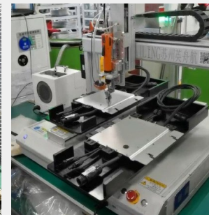
Automatic screw locking robot, to reduce workers' labor intensity
